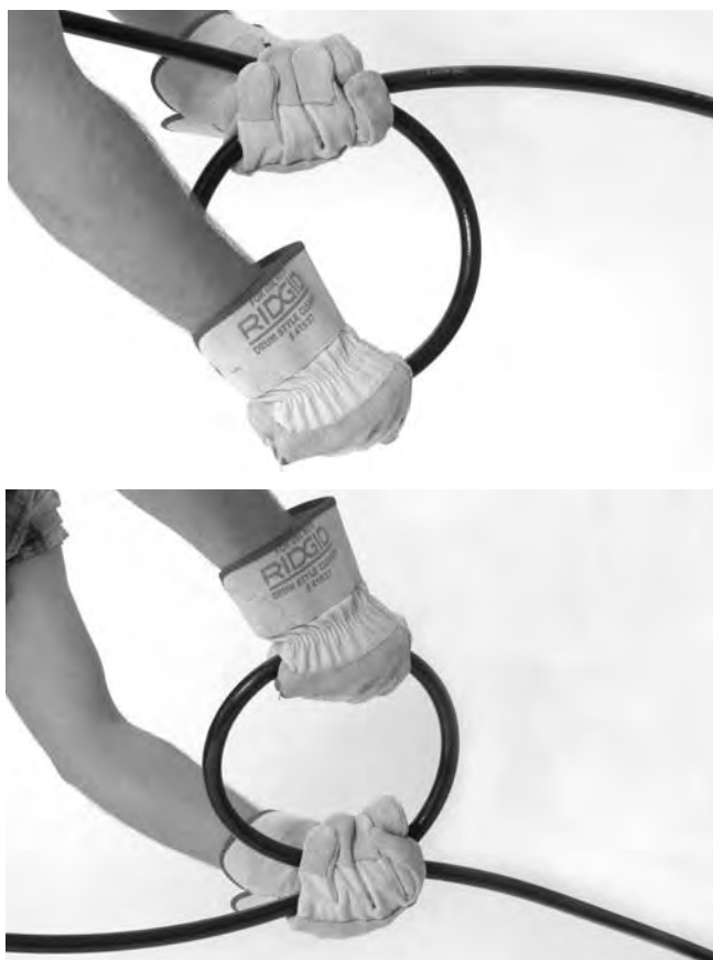
Figure 15 – Rotation du tuyau haute-pressure
