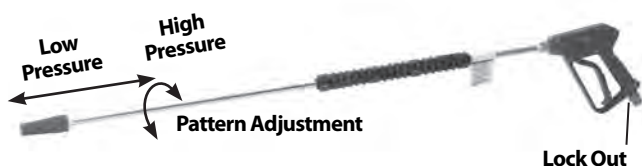
Figure 17 – Wash Wand Nozzle Adjustments
